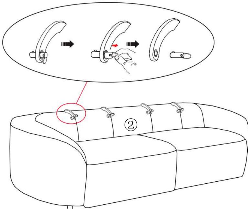
Step 2. Line up the holes of the metal rod with the holes of the back cushion and insert the pin to secure the back cushion in place.
